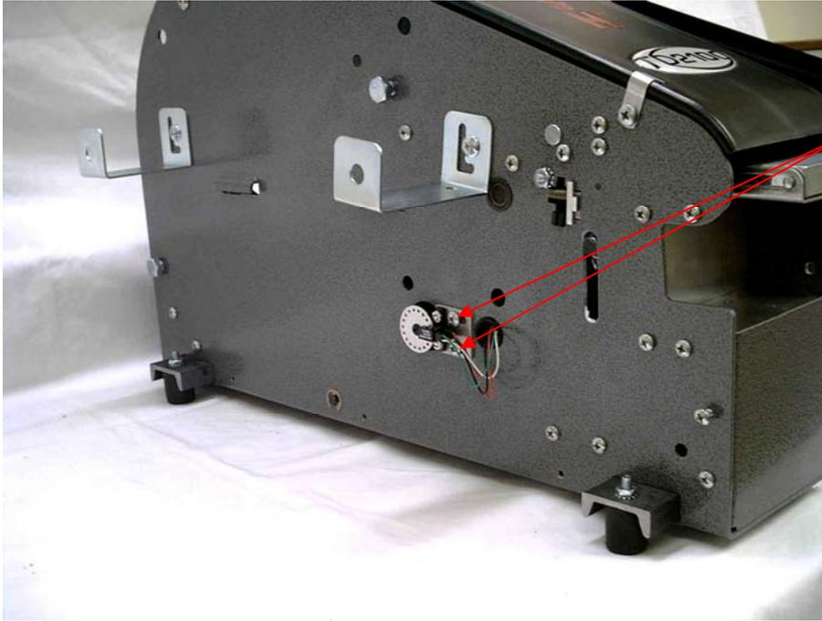
7. Facing the left side of the machine, with one hand hold the encoder remove the screws holding the encoder.
