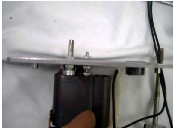
13. Looking at the outside surface of the gearbox/motor mount, attach the screws that are on the left hand side of the gearbox/motor mount tightly and the nuts on the right snugly
