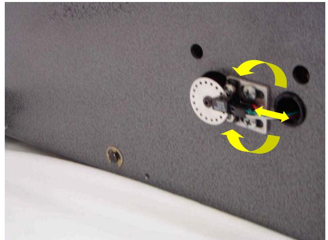
6. While moving the encoder forward, backward and at various angles, and keeping hands clear of the encoder wheel, run the machine at any given length until the machine is accurate within  $\pm 1/2$ ".
