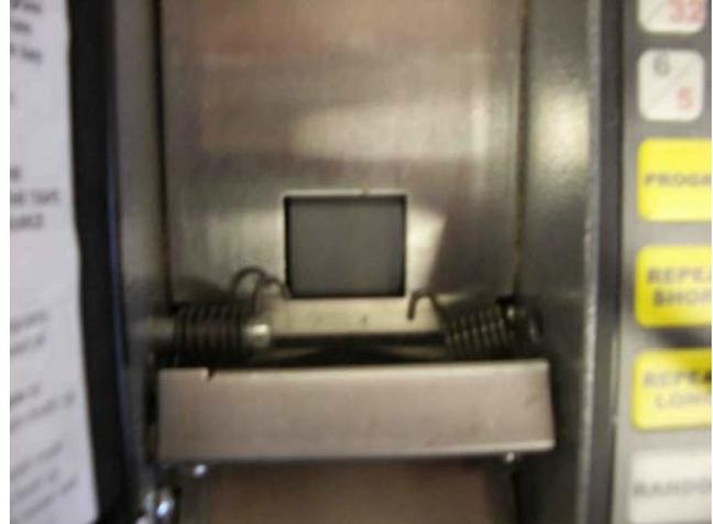
**Fig 13 Pinch Roller, Serial Numbers 601082 and Above**
