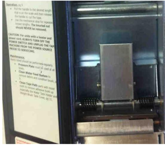
3. Facing the front of the machine, pull the pinch roller springs towards the front and to the left and right of the machine until the springs are no longer on the pinch roller.
