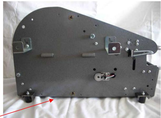
4. Slide the left side cover towards the bottom of the machine and pull the left side cover away.
