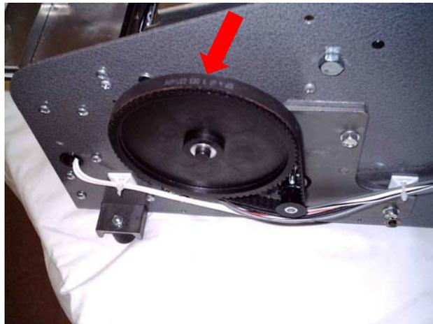
3. Facing the right side of the machine, remove the timing belt from the large timing pulley first, then from the small timing pulley.
