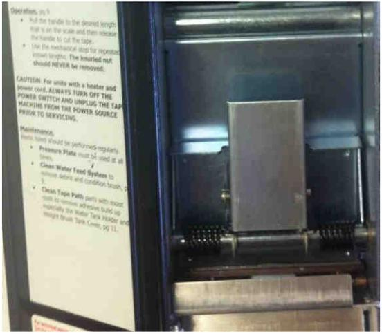
2. Remove the pressure plate.
