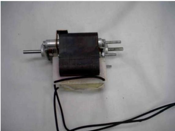
*NOTE: The motor is square when all of the plastic is touching the gearbox/motor mount.*
