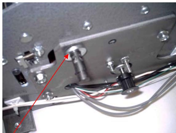
*NOTE: Make sure that any washers that were on the feed wheel shaft are now placed back on the feed wheel shaft.*
