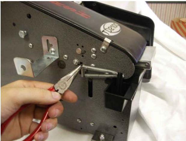
3. Use a pair of need-nose pliers to remove the springs that are attached to the blade shoe.
