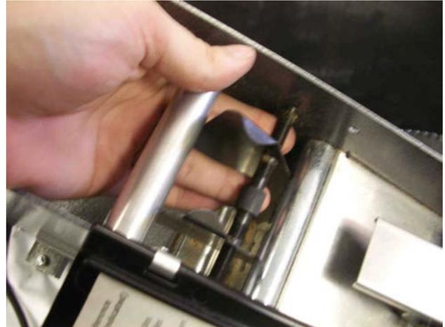
6. With the tape guides set towards the middle of the machine and one hand spreading the chassis apart, pull the turnbuckle to one side of the machine, twist the turnbuckle slightly and pull the assembly out the rear of the machine.
