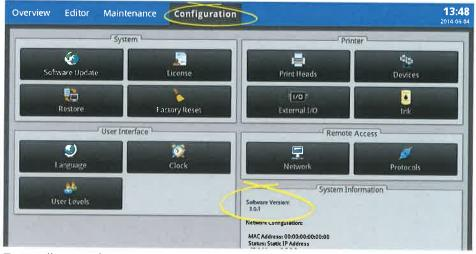
To install new software save an unzipped copy on to a USB memory stick and insert it into the MPERIA Controller USB port. Then tap the Software Update button, as shown above. When prompted to make a backup select **Yes**. Follow the displayed guide to complete both the backup and software installation.
