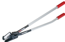
Model CU-25LH Part No. 0X-1528 Extra long handle cutter. Replaceable blades. Cuts strap through 2" x 0.050" (50.8 x 1.27 mm). Shipping weight: 8 lbs. (3.6 kg)
