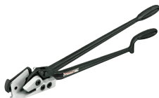
Model CU-25 Part No. 005740 For strap removal or cutting strap to length. Replaceable blades. Cuts strap through 2" x 0.050" (50.8 x 1.27 mm). Shipping weight: 8 lbs. (3.6 kg)
