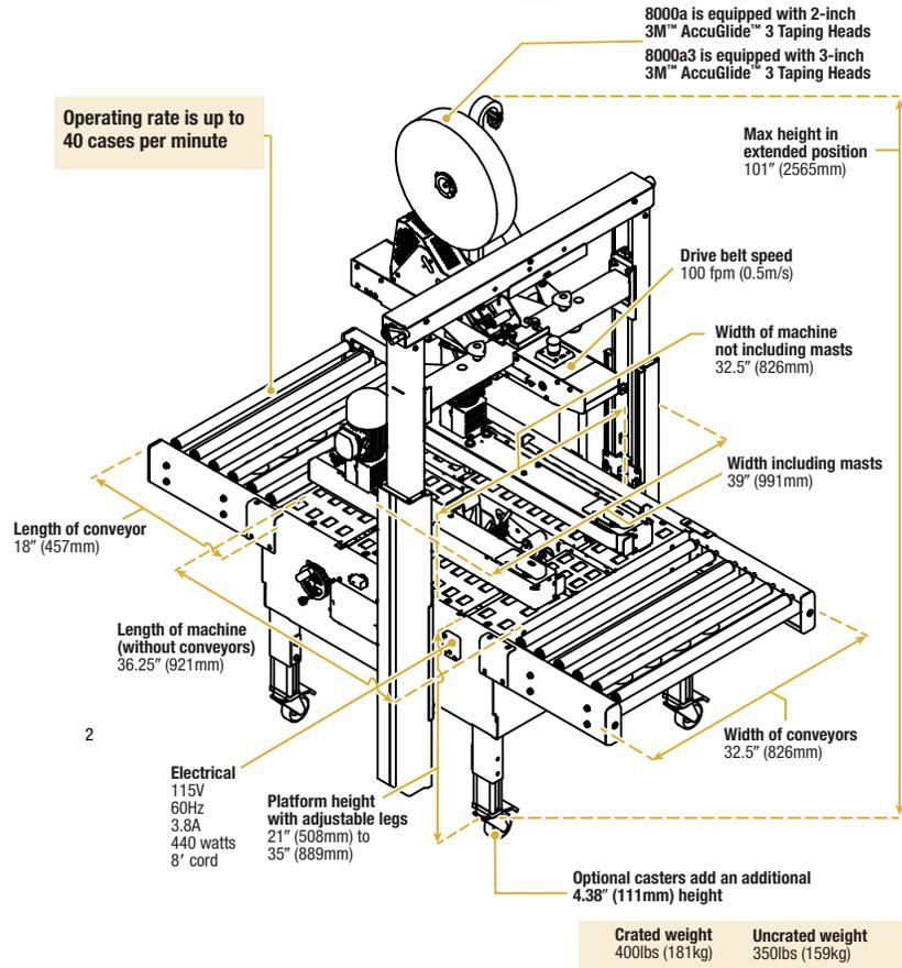
Box Dimensions for 8000a and 8000a3 Machines: Inches (mm)
